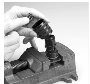
8. A receptacle shell mounted in the vise creates a good way to hold a plug during contact insertion.
