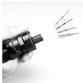
10. Place all cable hardware on cable before contact insertion.
