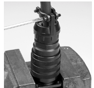
16. Tighten cable clamp securely.
