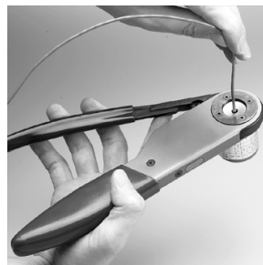
3. Crimp contact onto wire in one full stroke. The ratchet on the crimping tool will not release until the tool has completed a full stroke.
