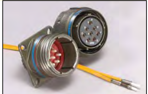
Single Mode Size 16 Fiber Optic Termini Designed for use in the size 16 contact cavities of Multi-channel MIL-DTL-38999 Series III Connectors and Amphenol CF-52 & CF-50 Fiber Optic Connectors
