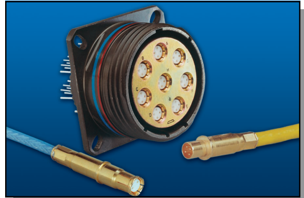
D38999 Series III Groundplane Connector with Quadrax PCB Sockets Installed Contacts front are Differential Twinax (left) and Quadrax (right)
