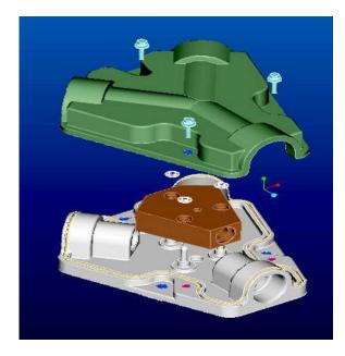
The second solution offered by Amphenol is called the "Amphenol Y" Connector. This connector is a unique packaging solution consisting a molded base plate, a copper "connector", and a molded top cover. When attached to the traction motor, this unit creates a safe, reliable, and efficient means of conducting high amperage current from the third rail or catenary to the propulsion controller. Each "leg" of this assembly can safely accommodate up to 1000 amps through the 18mm RADSOK contacts.
