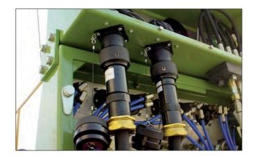
Starline EX offers a full range of hardware styles including the use of EX rated cable glands, mechanical clamps and gland nuts.
