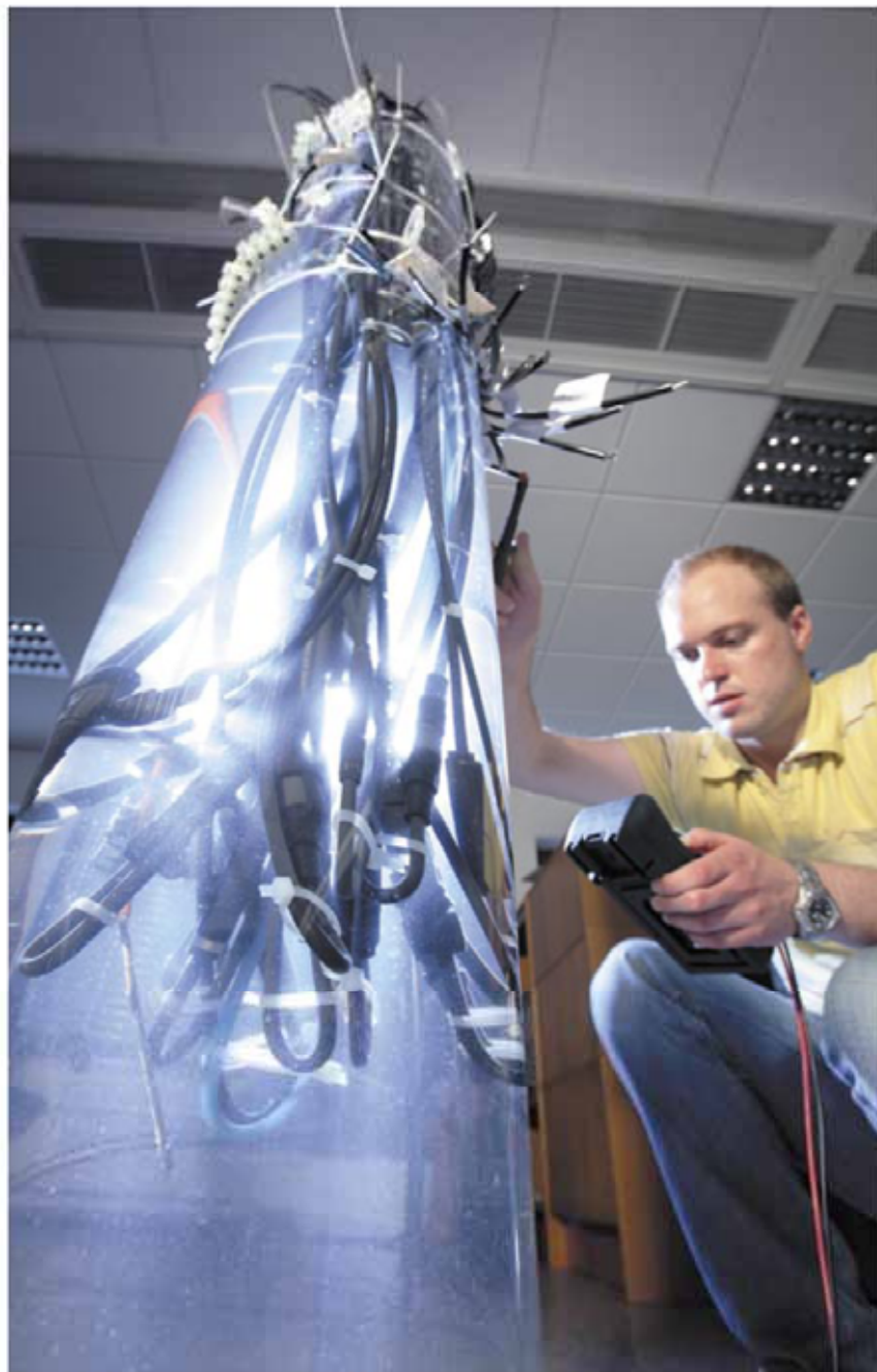
19 PV connectors in a 1 m deep water bath for three weeks: That's one way PHOTON Lab tested each connector's stamina. Pictured here is lab engineer René Düpont.
