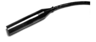
The H507A wide band (10 Hz to 100 kHz) hydrophone is a very small, high-sensitivity device incorporating an ultra-low noise preamplifier (-166 dB re  $1V/\sqrt{Hz}$  at 10 kHz) and a circuit for the insertion of an electrical calibration signal. In addition, the preamplifier can drive up to 200 meters of cable. The sensor and amplifier are electrostatically shielded and molded in hydrolytically stable, void free polyurethane.
