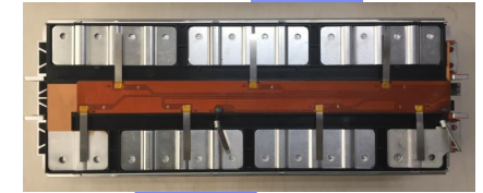
Battery Sensing Covers (CCS) /Wiring, busbar with temp and Cell voltage measurement
