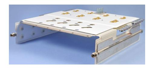
Integrated liquid cooling piped
