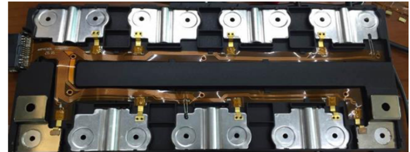
Busbar integration of sensors
