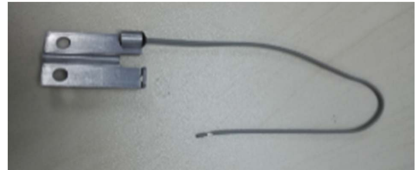
Busbar integration of sensors
