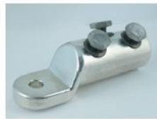
C400 x 16 AL2 SW19 - installation tool size (6-8 allen key size) - 13-24 outer heagren size - conductor material and class acc. DIN EN 60228 - palm hole size - conductor cross-section - C = lug series
