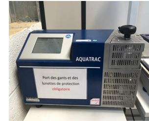
%H tester for plastic raw material (AQUATRAC)
