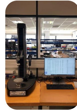
Traction control machine for insertion/extraction force for pins, test of the US welding...
