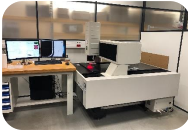
Tri Dimensional Machine by sensor and camera (Microvu)
